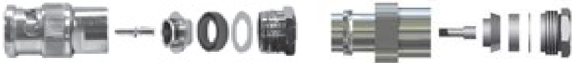
Figure 2 - CF-F & CF-E kits are recommended to only be used with 0.25 in diameter cable. Smaller cable diameters and/or foil or braided shields will not hold the cable firmly.
